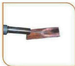
Step2.Bake the material to be welded to remove moisture and oil.
