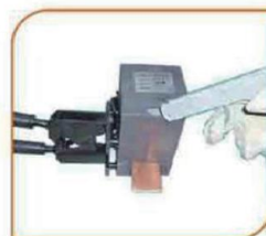
Step6.To use the ignition gun to ignite the powder, the person must stand on the side of the mold mouth.
