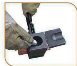
Step4.Put in spacer to seal the flow guide
