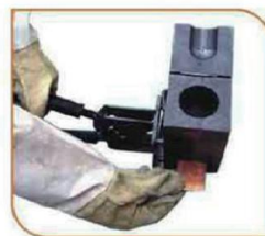
Step3.Place the material to be welded into the mold and tighten the mold.
