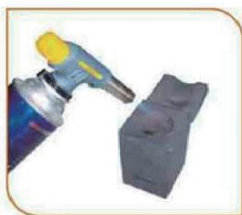
Step1.Bake mold to remove moisture.
